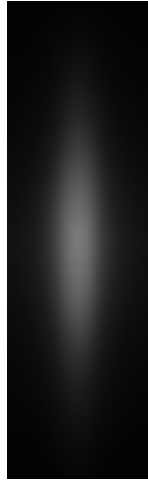
Figure 5.1.2: Elliptical shape of the beam acquired by the DCC1545M webcam.
