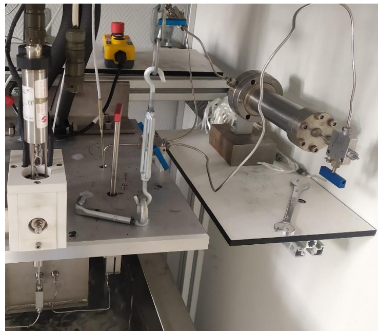
Figure 68. Details of the VTD test rig including the variable volume cylinder, pressure transducers and the thermostatic bath
