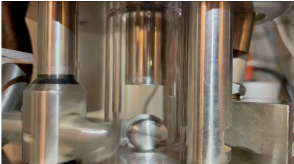
Figure 70. Picture of the variable volume cell at CTP (Mines ParisTech) loaded with the \text{CO}_2+\text{SiCl}_4 mixture in liquid phase
