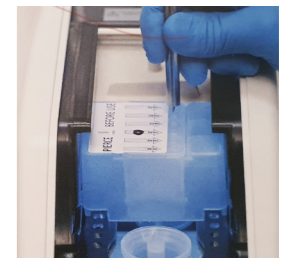
Fig. 2-15 Piercing of the liquid tank of tooth transformer device
