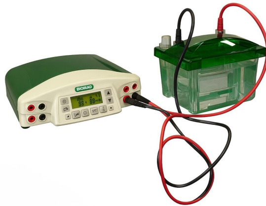
Figure 2.3 SDS-PAGE electrophoretic cell with power supply.
