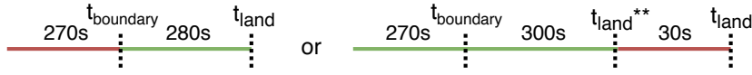
Figure 5.4: The s/c touches the surface at t_{land} . The surface can be reached before t_{land}^{**} \equiv t_f (left) or after (right). Red: control off. Green: control on.
