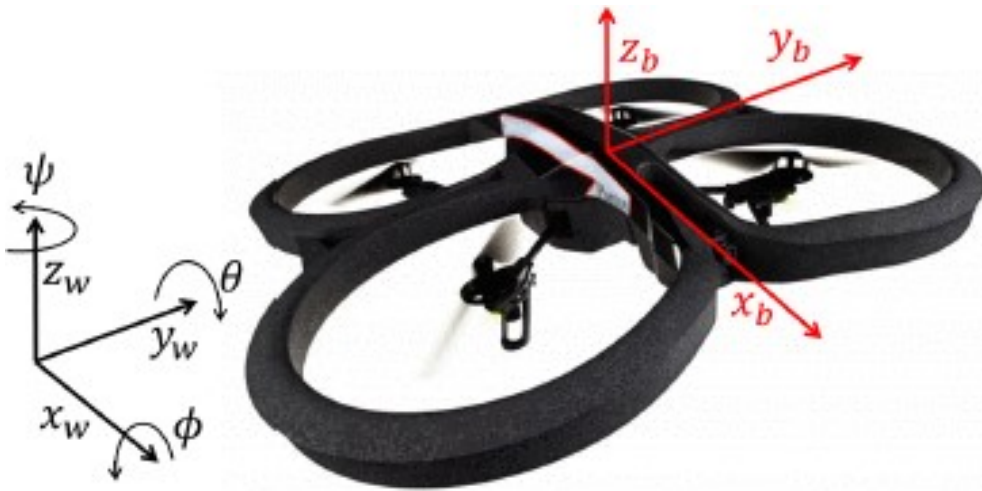
Figure 2.5: Coordination frames with respect to the AR.Drone
