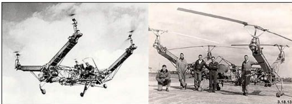
Figure 1.3: Convertawings Model "A" Quad-copter
