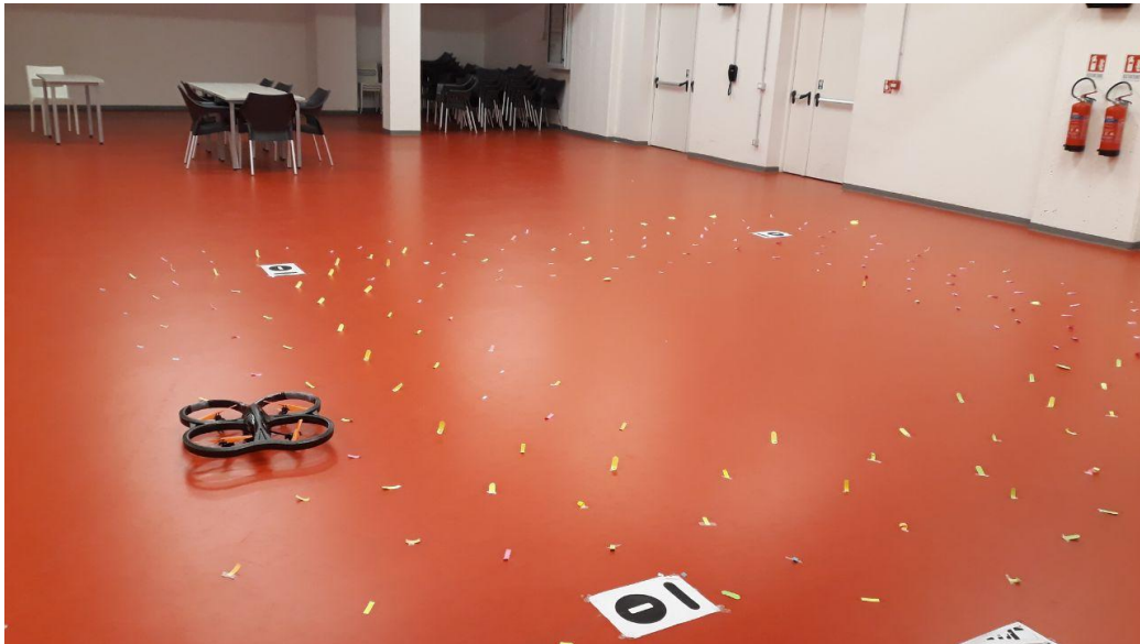
Figure 6.6: The test path prepared in an auditorium. The floor texture is increased with colored stickers for the sake of vision estimated velocity
