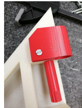
Figure 4.36: Hinges are screwed in tassel
