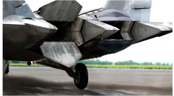
Figure 5.5: F16's single-engine afterburner, which cannot provide thrust vectoring. Figure 5.6: F22's thrust vectoring nozzels.
