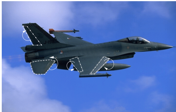
Figure 5.4: Main aircraft control surfaces and their typical deflection directions.
