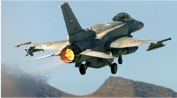
Figure 5.5: F16's single-engine afterburner, which cannot provide thrust vectoring. Figure 5.6: F22's thrust vectoring nozzels.
