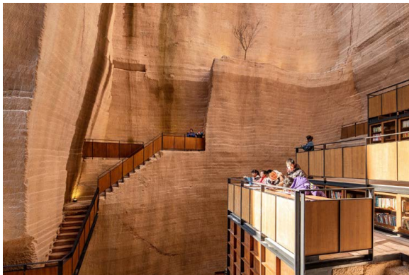
Figure 479. Figure x Quarry No. 8 A clear visual distinction is made between the “found” context (rough, hand-hewn stone walls) and the “inserted” architecture (precise, warm bamboo shelving and steel railings). Source: DNA Design and Architecture
