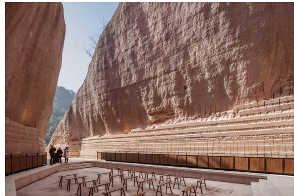
Figure 481. Figure x Quarry No. 9 The performance space utilizes the porous volcanic rock walls as natural acoustic absorbers, eliminating the need for artificial soundproofing materials.. Source: DNA Design and Architecture
