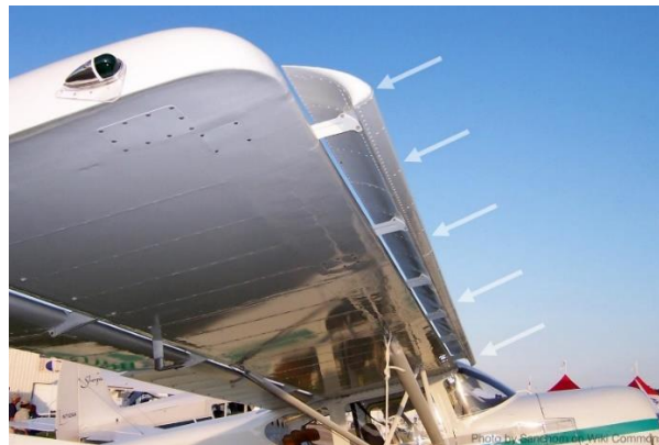
Figure 2.1 : Example of movable slat on a wing of an aircraft
