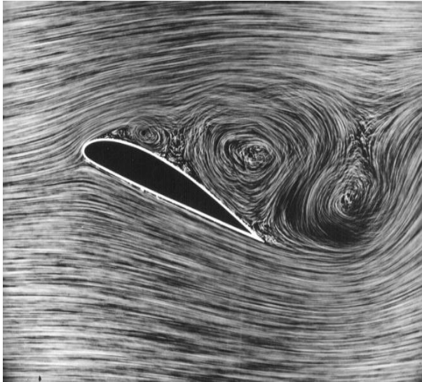
Figure 1.8 : Flow structure of airfoil stall
