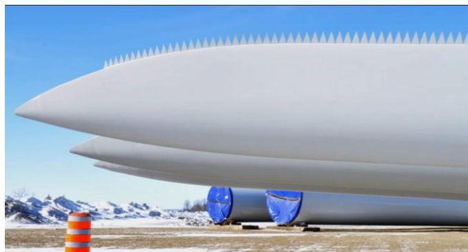
Figure 2.7 : Serrated trailing edge of wind turbine blade
