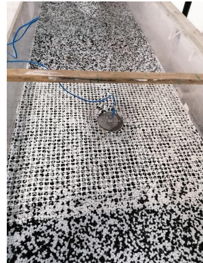
Figure 84. Photograph bed surface after protected area test 1-M
