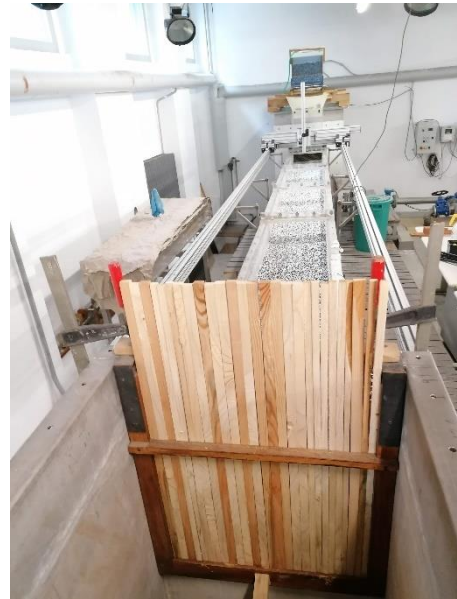
Figure 26. Photograph of sticks as a boundary condition at the end of the channel
