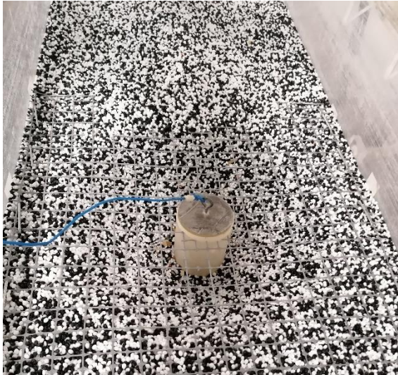
Figure 99. Photograph scour surface close the Pier test 1-XL
