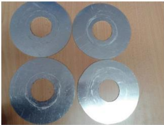
Figure 14. Photograph of aluminum collar used in reference [18]
