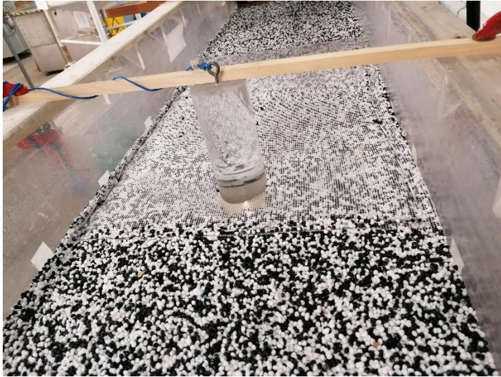
Figure 79. Photograph scour surface close the Pier test 4-S
