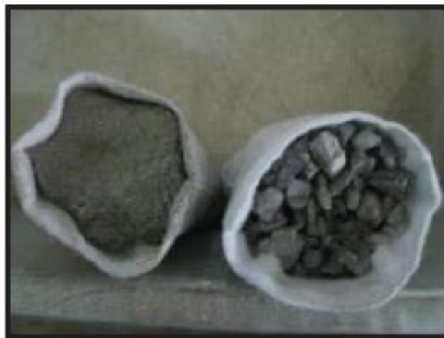
Figure 19. Geotextainers with fine crushed concrete and coarse crushed concrete [19]
