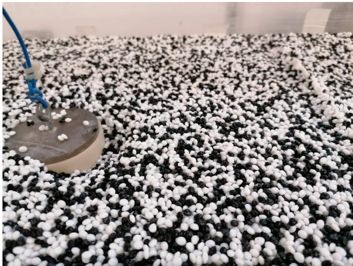
Figure 67. Photograph scour surface close the Pier test 1-S
