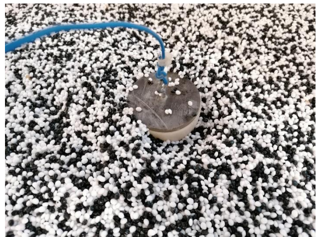
Figure 51. Photograph scour hole - test 1-S
