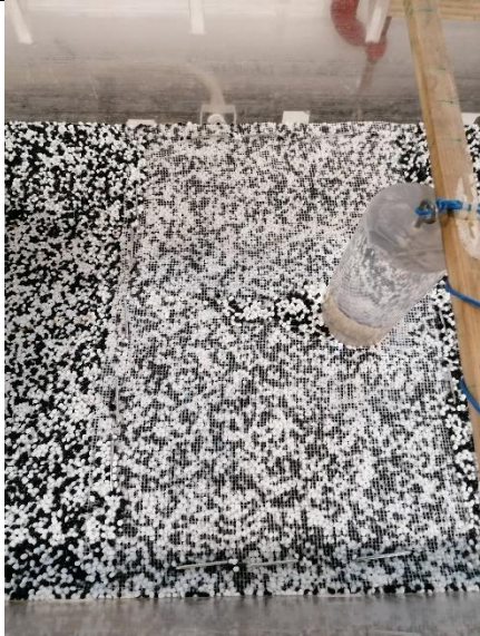
Figure 75. Photograph scour surface close the Pier test 3-S
