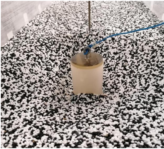
Figure 50. Photograph scour hole- unprotected test
