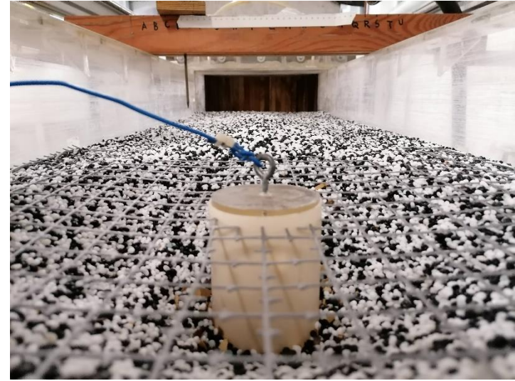
Figure 100. Photograph bed surface after protected area test 1-XL
