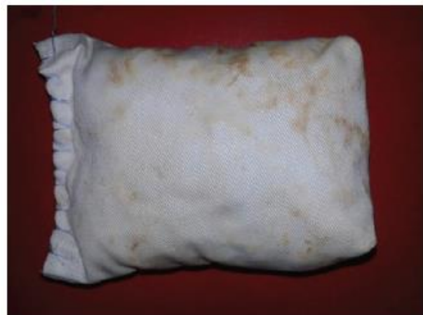
Figure 17. Photograph of geocontainers with crushed concrete containing oil pam shell used in reference [18]
