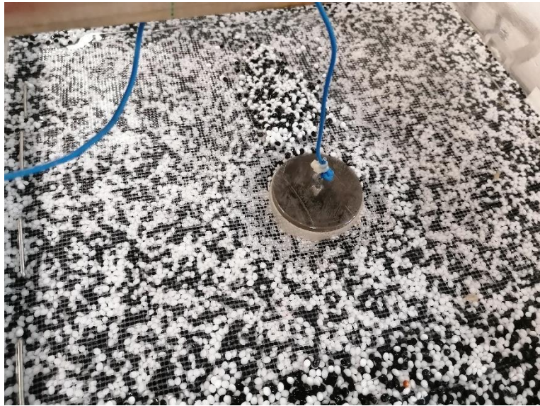
Figure 71. Photograph scour surface close the Pier test 2-S
