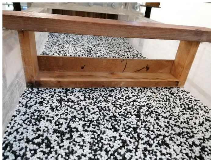
Figure 27. Device to straighten the bed
