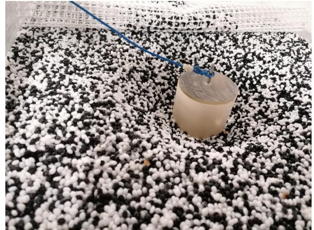
Figure 53. Photograph scour hole - test 4-M
