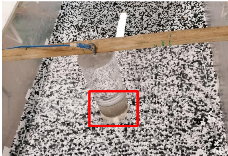
Figure 62. Photograph weak area between pier and net
