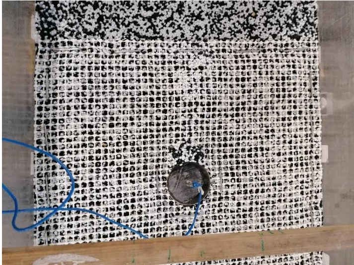
Figure 83. Photograph scour surface close the Pier test 1-M
