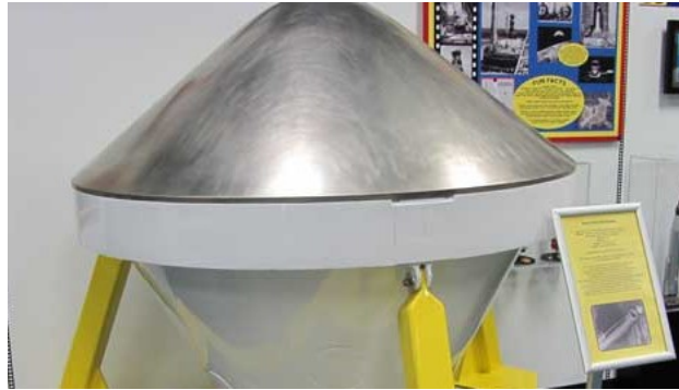
Figure 28 – A Mark 2 re-entry vehicle copper heat sink on display [41].
