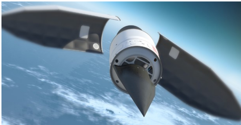
Figure 19 – Rendering of the HTV-2 attached to an upper stage [26].
