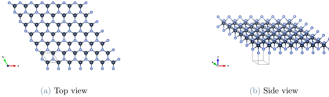
Figure 2.1: Sketch of monolayer \text{WS}_2 crystal structure: tungsten atoms in dark blue, while sulfur atoms in light blue
