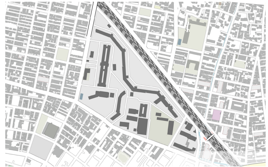
Figure 1.33 Site Plan for Kawaguchi Shibazono Danchi, 1978. It has its shape to act as a firewall to protect the city in the west side from the noise of the railways. This becomes an icon by itself. Source: Map by Authors
