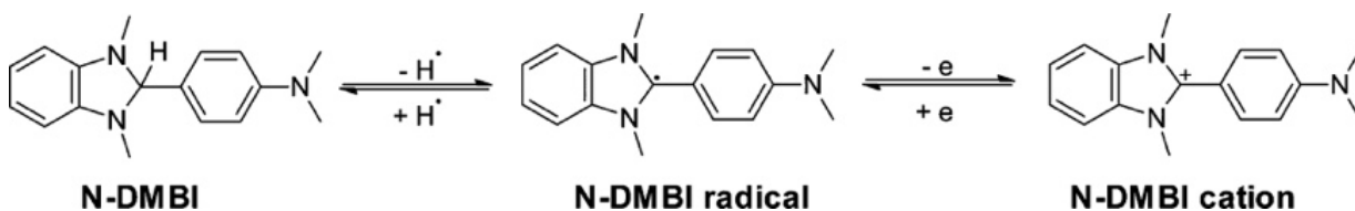
Figure 2.2: Hypothesized mechanism for n-type doping, composed of 2 steps, a hydrogen transfer followed by an electron transfer. 59
