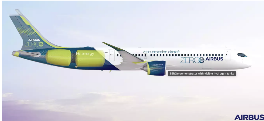
Figure 1.5: A possible tank integration into the airframe ( www.airbus.com )
