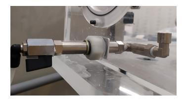
Figure 3.20. Detail of the hydraulic connection in the upstream reservoir
