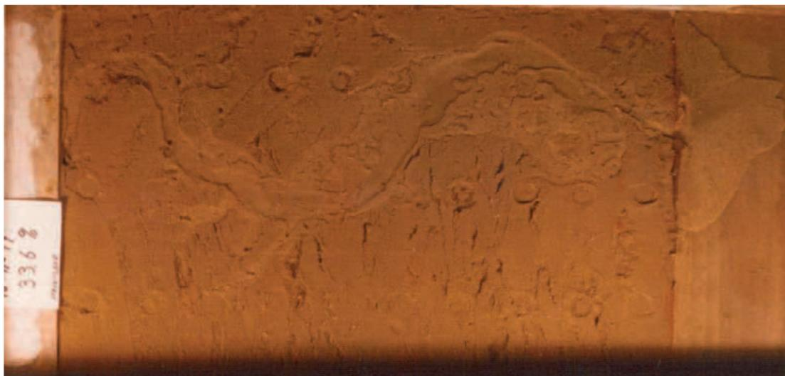
Figure 1.2. Pipe development in laboratory tests (Van Beek, Knoeff, et al. 2011)
