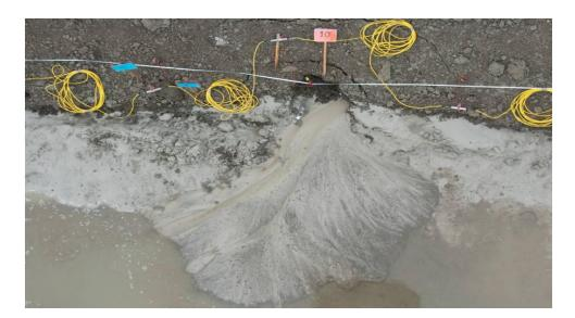
Figure 2.24. Widening of the channel with a consequent increase in the eroded material (Van Beek, Knoeff, et al. 2011)
