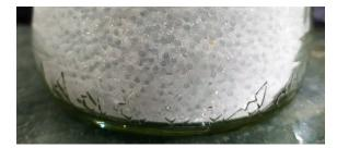
Figure 4.8. No separation observed on the compacted sample in wet condition
