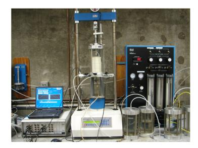
Figure 2.12. Suffusion experimental triaxial cell (Xiao and Shwiyhat 2012)
