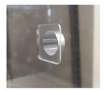
Figure 3.14. Hole with cavity for the positioning of the squared screw head
