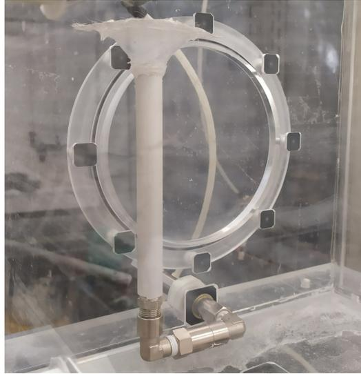
Figure 3.22. The continuous overflow system
