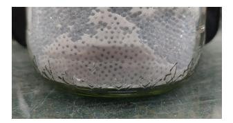
Figure 4.7. Effect of grain separation of the fine and medium particles from the coarser ones for highly compacted samples
