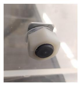
Figure 3.15. Grey screw bolted with a white nut and with the addiction of a circular silicon protection gasket
