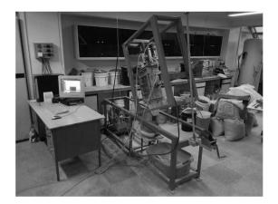
Figure 2.2. Overview of the tiltable apparatus developed for internal erosion studies (Pachideh and Hosseini 2019)
