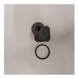
Figure 3.17. Cavity on the screw and its O-Ring
