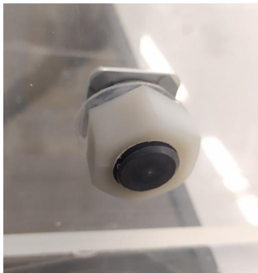
Figure 3.15. Grey screw bolted with a white nut and with the addition of a circular silicon protection gasket
