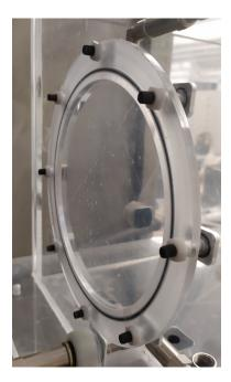
Figure 3.7. Detail of the removable cap with its O-Ring put in place
