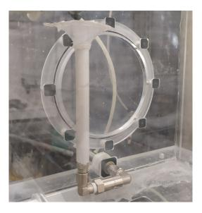
Figure 3.22. The continuous overflow system
