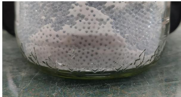
Figure 4.7. Effect of grain separation of the fine and medium particles from the coarser ones for highly compacted samples
