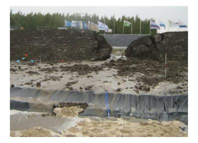
Figure 2.25. Collapse of the levee (Van Beek, Knoeff, et al. 2011)
