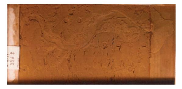
Figure 1.2. Pipe development in laboratory tests (Van Beek, Knoeff, et al. 2011)
