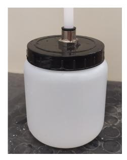
Figure 3.23. Trap box employed for collecting the eroded material
