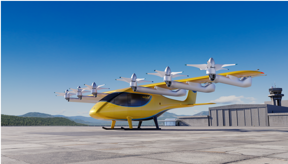
Figure 2.3: Wisk Aero Generation 6 eVTOL, an example of a winged lift-and-cruise architecture developed for Advanced Air Mobility operations.
