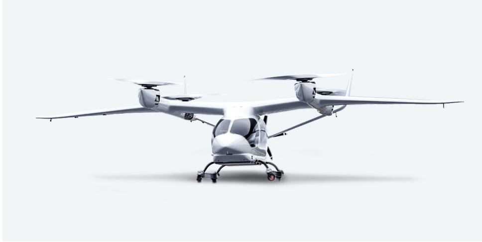
Figure 2.4: BETA Technologies ALIA lift-and-cruise eVTOL concept, showing separate vertical lift propellers and a dedicated rear cruise propeller.
