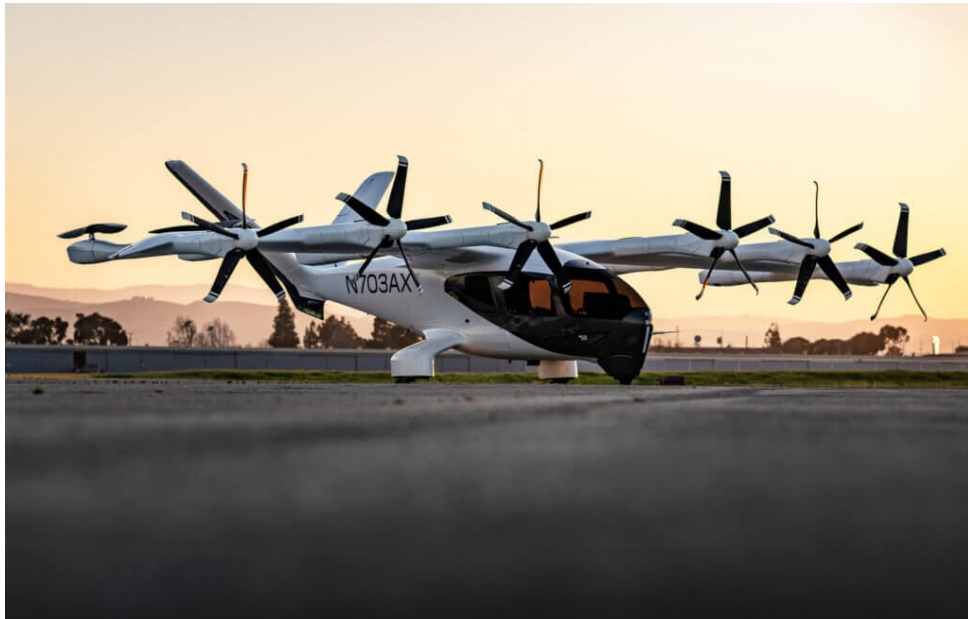
Figure 2.7: Archer Midnight eVTOL aircraft, an example of a winged distributed-propulsion configuration designed for Advanced Air Mobility operations.
