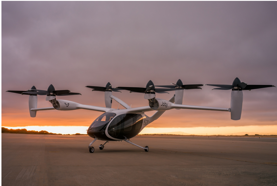
Figure 2.6: Joby Aviation S4 vectored-thrust eVTOL concept, featuring tilting electric propellers for vertical take-off and efficient wing-borne cruise.
