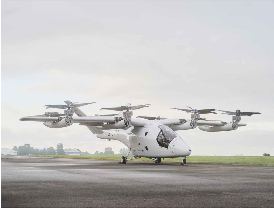
Figure 2.8: Vertical Aerospace Valo/VX4 eVTOL concept, based on tilt-shift propellers to combine vertical flight capability with fixed-wing cruise efficiency.
