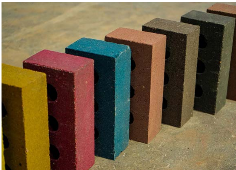
Figure 4: bricks made of construction waste by Kenoteq
