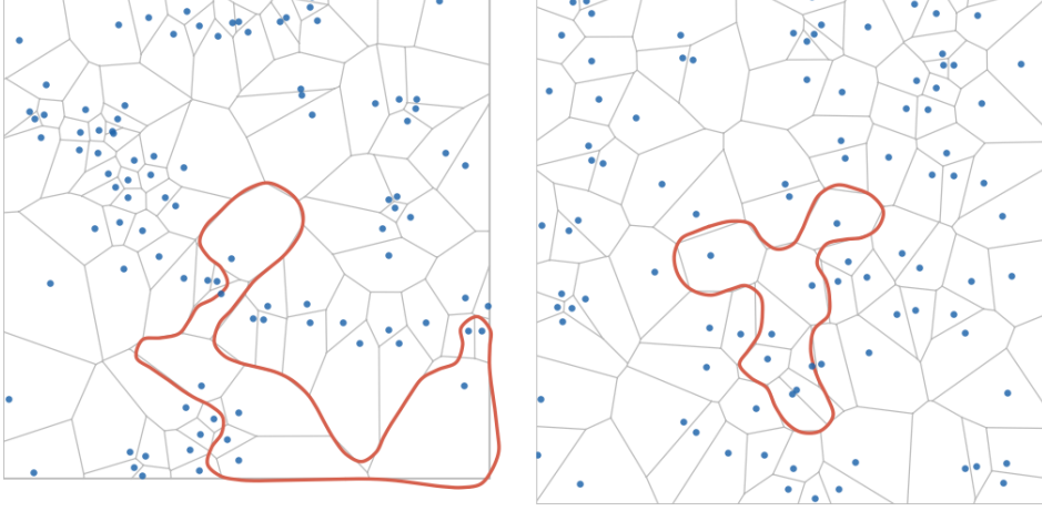
Figure 3.3: Two generated track lines after cell selection and smoothing steps, simplex noise (left) uniform (right); the simplex noise based generation displays its potential of generating large straight sections in sparse areas, whilst cluster enforce a winding topology.
