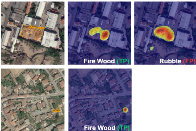
Figure 3: Examples of images of the test set and corresponding predictions performed by the selected model. In the first case, the model correctly predicts Fire Wood focusing on the right aspects but it also predicts Rubble due to inter-class similarity. In the second case, the model can correctly predict a small instance of Fire Wood .
