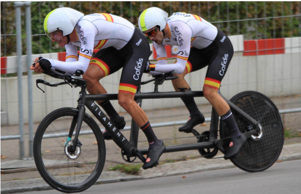
Figure 3.4: The Spanish Tandem team adopted a different position, with the stoker placing his hands on aero bars rather than gripping the frame. Credit: Davide Andreoli.
