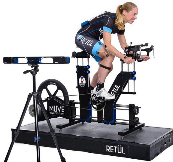
Figure 2.4: Modern laser systems are nowadays used to measure the athlete's body angles, due to the importance of a correct bike fitting. Credit: Retul.
