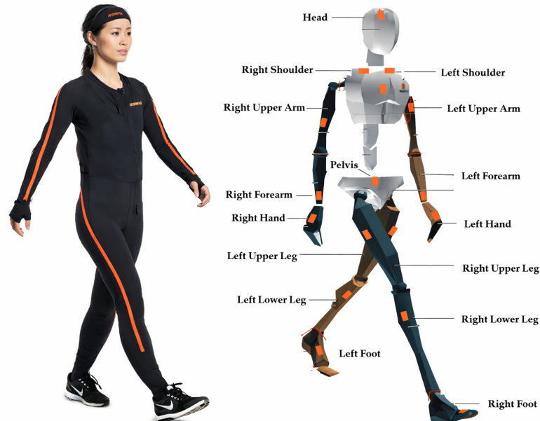
Figure 4.3: Xsens sensors placement on the body. Credit: Xsens.
