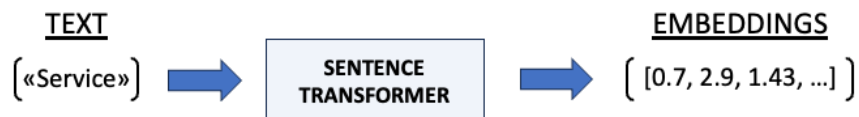
Figure 4.1: General view about how a Sentence Transformer works: it takes some text and it converts it into an array of values.
