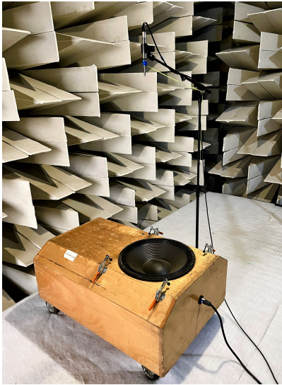
Figure 9: SPL measurement in anechoic room with a free-field pressure microphone.
