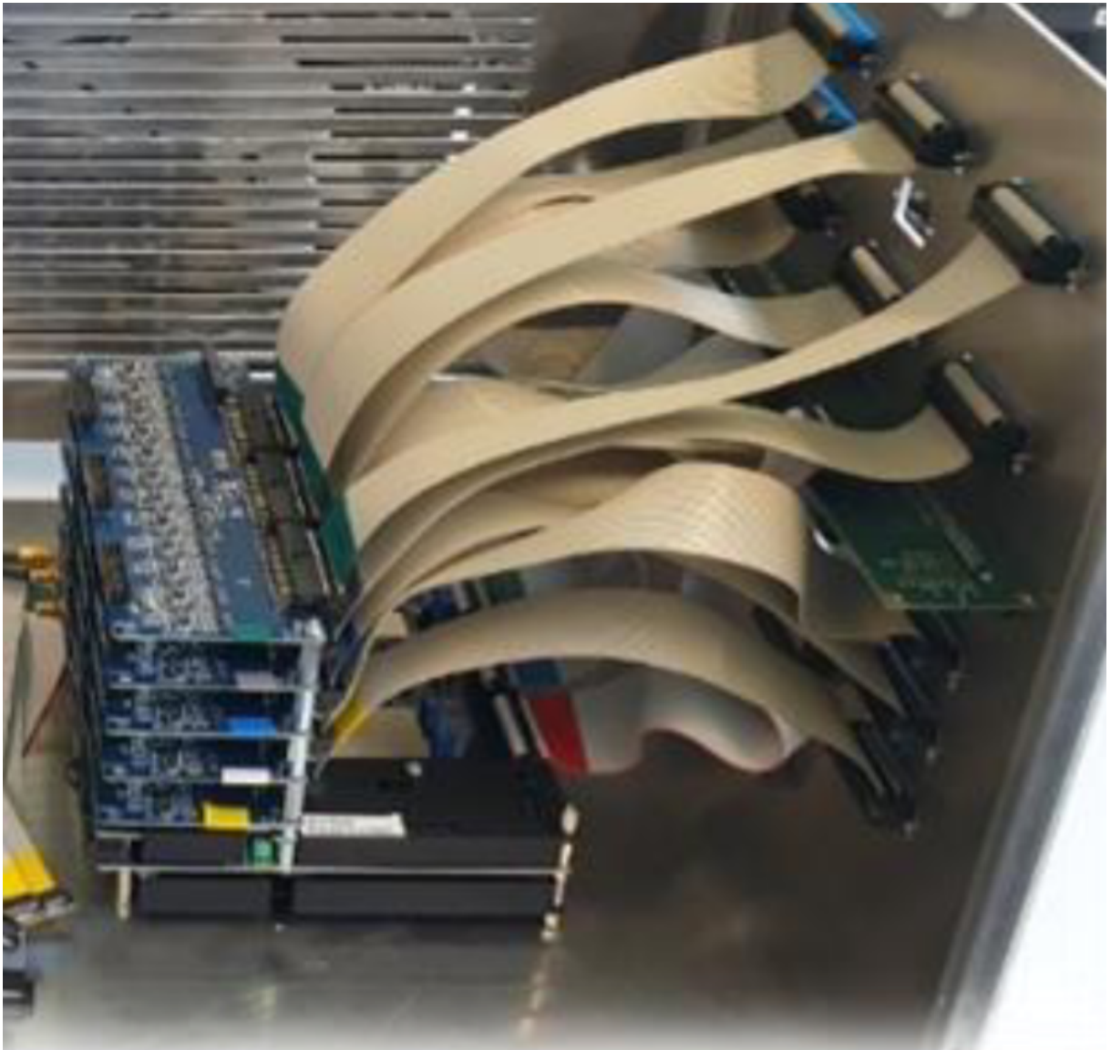
Figure 2.40: Bias Board developed by XGLab, structured for the 166 pixel detector setup (photo coming from the MPP 166 pixel setup presentation).
