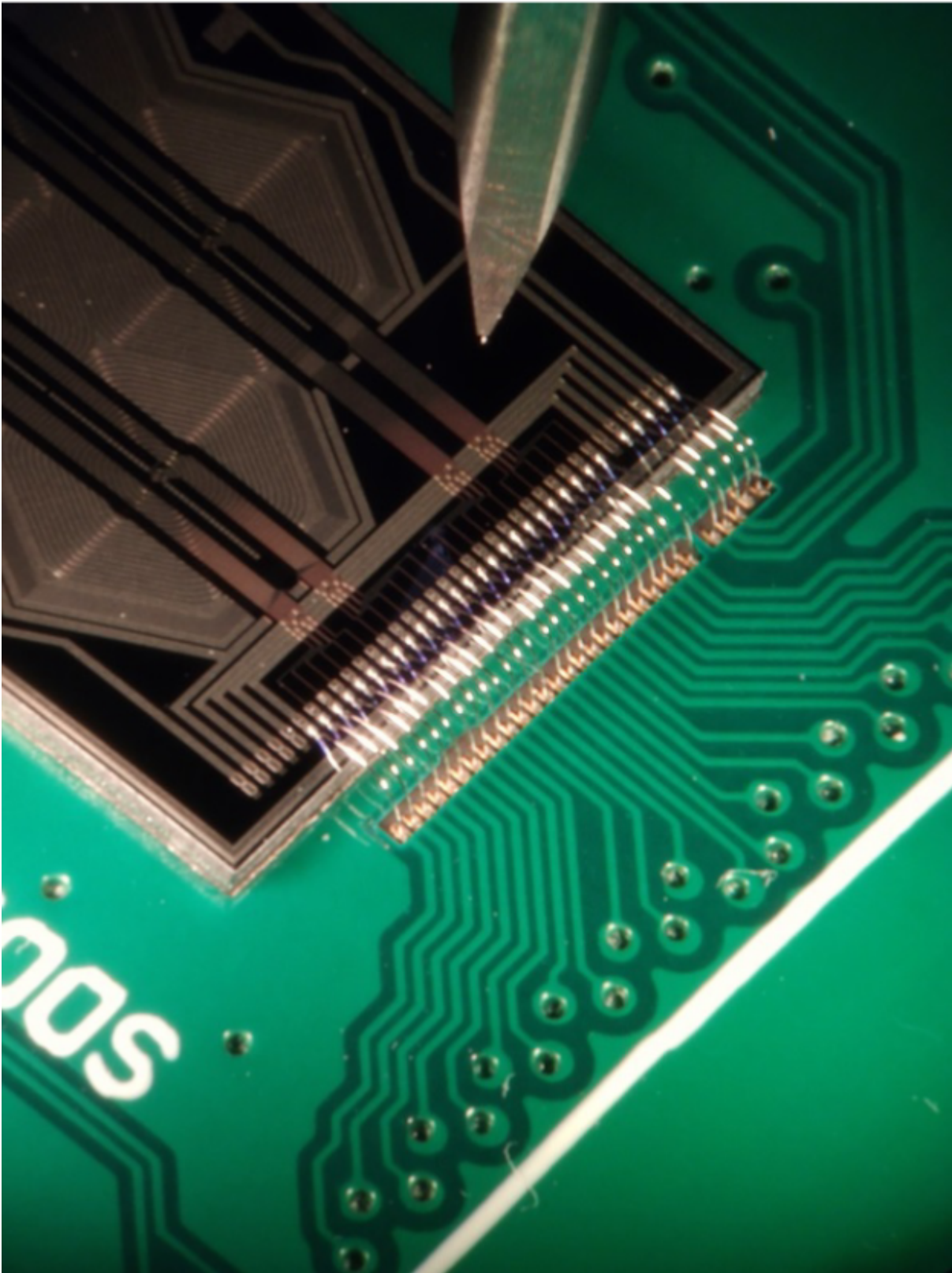
Figure 2.12: Picture of a zoomed wire bonding part of the detector board with the 12 pixel SDD[4].
