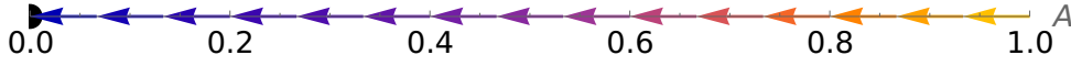
Figure 2.4: Dynamics of the DSVM system with parameters z_A = 0 , q = 0.8 and z_B = 0.2 . The arrows show the convergence of A(t) towards the two stable points, colored in black.
