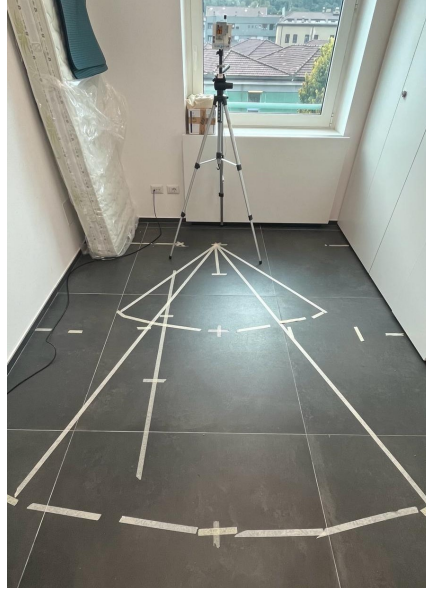
Figure 4: Target positioning in the test environment.
