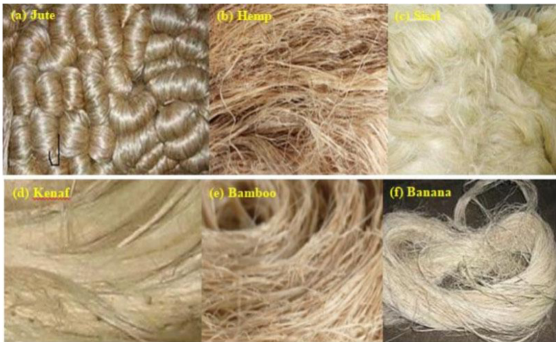
Figure 2.1: Commonly used natural fibers [3]: (a) jute; (b) hemp; (c) sisal; (d) kenaf; (e) bamboo; (f) banana.
