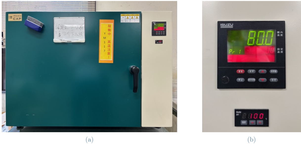
Figure 3.5: Drying equipment used for conditioning: (a) dryer unit; (b) temperature control panel.
