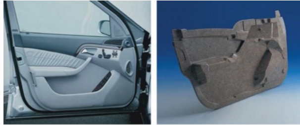
Figure 2.7: Automotive sector [23]: composite door panel of S-Class Mercedes-Benz.
