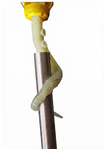
Figure 3.8: Arm with active suckers grasping a cylindrical object (20mm diameter). Reprinted from [43].
