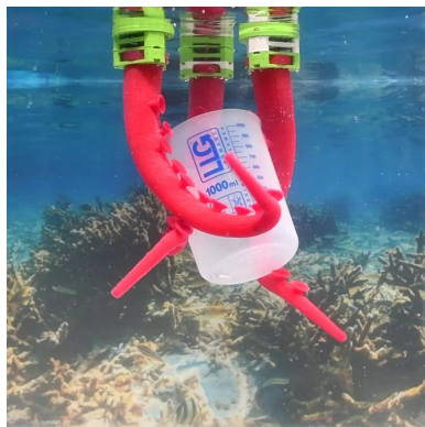
Figure 7.7: Example of "buckling out of the bending plane" phenomenon. The arms suddenly twists sideways instead of compressing the target, resulting in a failed grasp.
