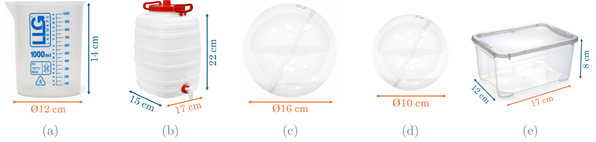
Figure 7.6: Set of objects used for the experimental grasping tests: (a) becher, (b) barrel, (c) large sphere, (d) small sphere, and (e) box. For each object, the dimension highlighted in orange represents the characteristic length ( L_c ), defined as its horizontal width.
