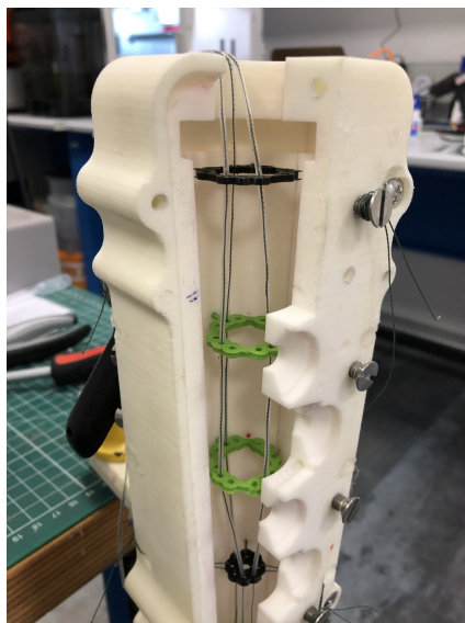
Figure 5.3: The mould during insertion of the internal supports; type 1 supports are shown in green and type 2 supports in black.
