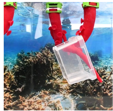
Figure 7.8: Successful shape-grasping configuration performed by a single arm to sustain the rectangular box.
