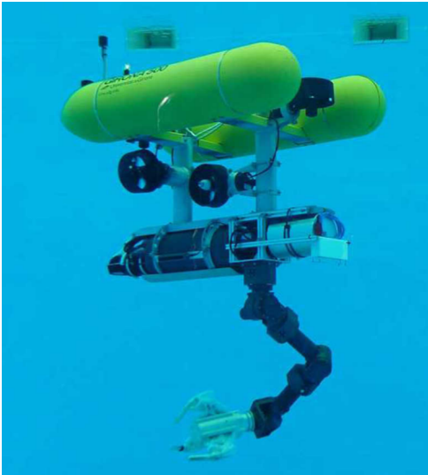
Figure 3.1: The Girona 500 AUV platform with its arm and gripper. Reprinted from [5].
