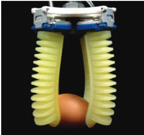
Figure 3.5: Soft Bionic gripper with variable effective length, grasping an egg. Reprinted from [23].
