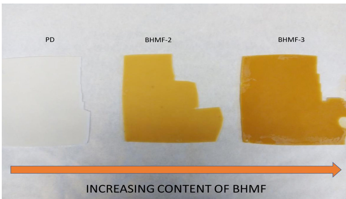
Figure 29 Resulting films from molding process. From left to right PD, BHMf-2, BHMf-3.
