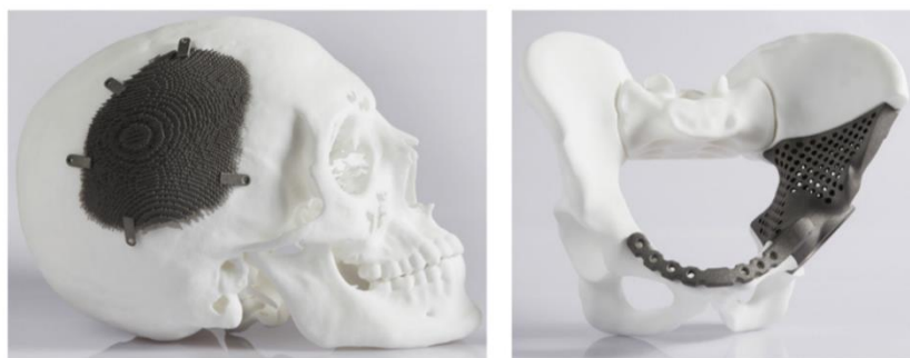
Figure 1.4: Titanium implants for the skull (left) and pelvis (right) produced using an EOSINT M 280. (Thompson et al. , 2016).
