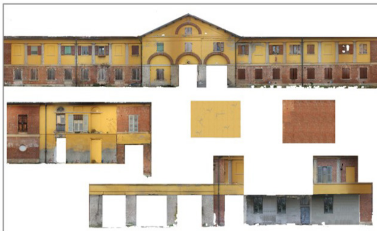
Fig40. The transformation of 2D heritage information from site photo (top), orthophoto (middle) and texture map (bottom)
