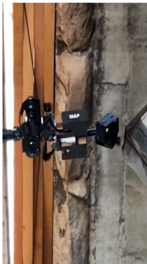
Rails to carry the photogrammetry camera
