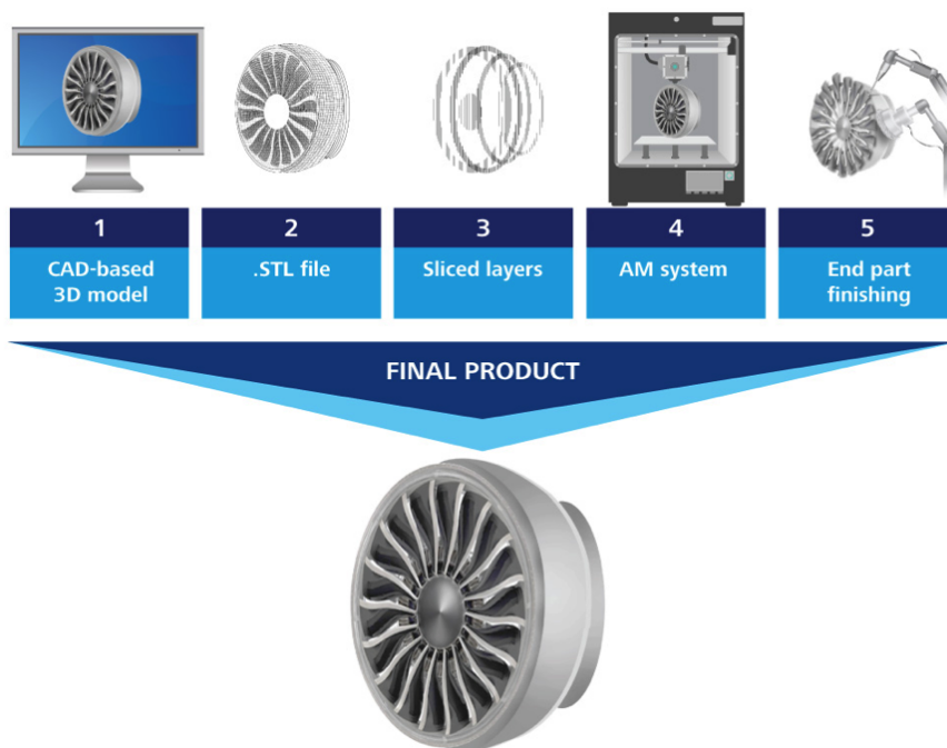
Figure 1.14: Steps in the fabrication of an AM part (from [66]).
