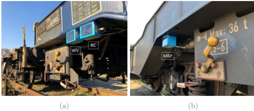
Figure 10: Position of sensor nodes on Breaking Valve (BC), Braking Main Pipe (BMP) and Weighting Valve (WV)
