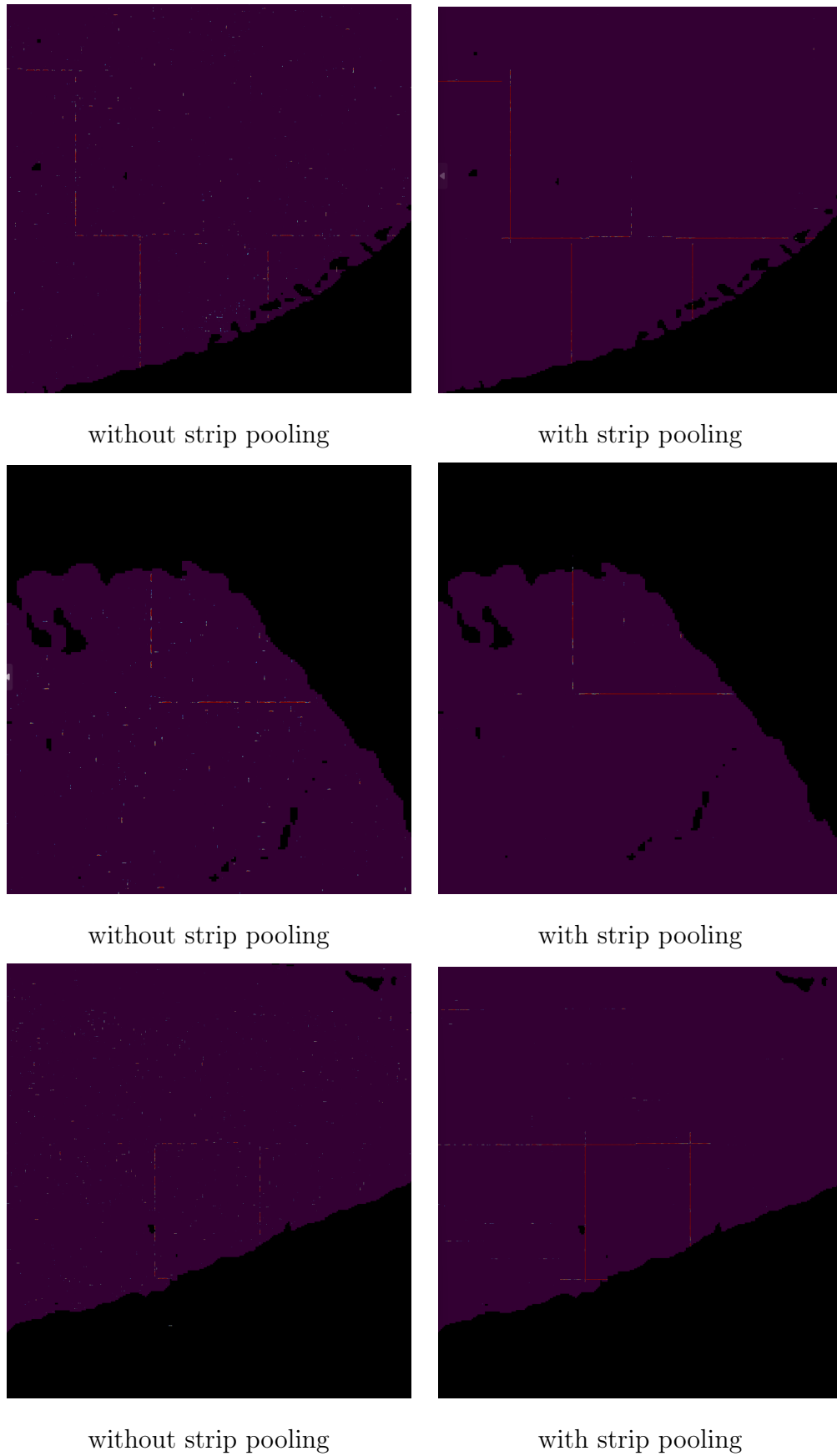
Figure 5.16: Impact of strip pooling on the raw logits predicted by the stitch detection branch.
