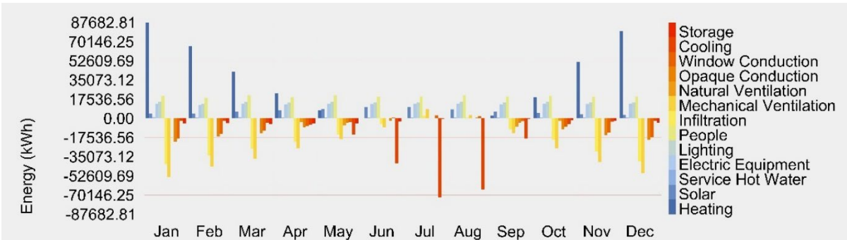
Figure 5-105 Monthly thermal load balance including balance_stor, illustrating the effect of thermal mass on heat storage and release alongside major heat gains and losses.
