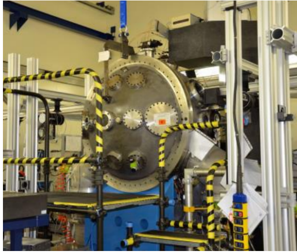
Figure 1.9: Closed chamber. This is where the target is placed (ENEA archive).
