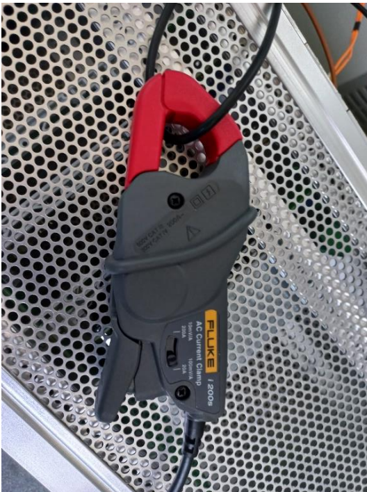
Figure 3. 7: AC current clamp and its accuracy range
