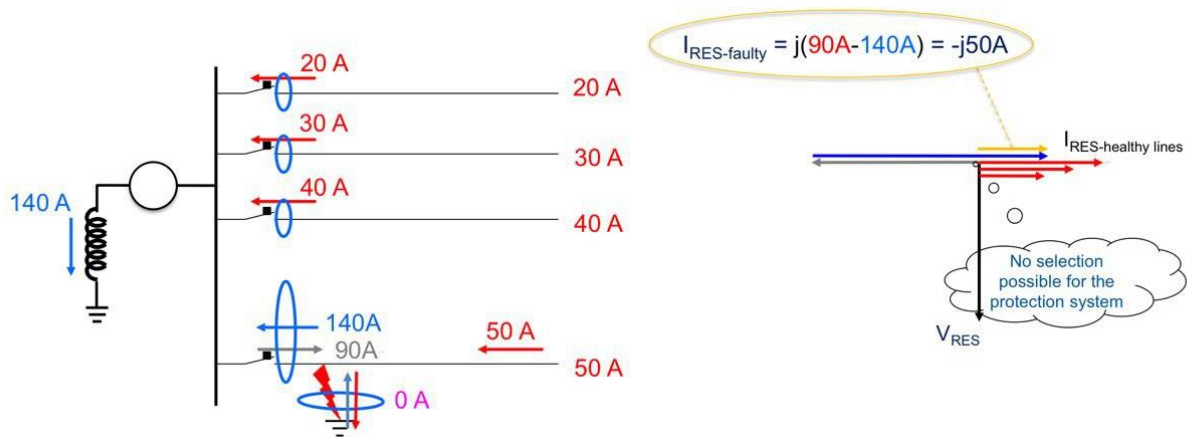
Figure 1.9: Case of compensated MV network with a pure Petersen coil[1]
