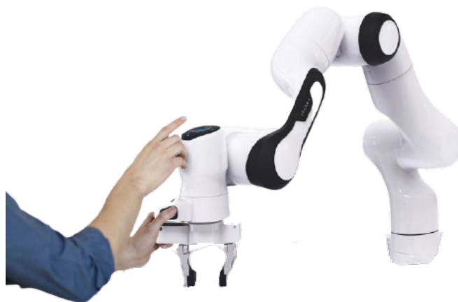
Figure 2.2: Cobot FRANKA EMIKA moved by an operator through the pressure of a dedicated button
