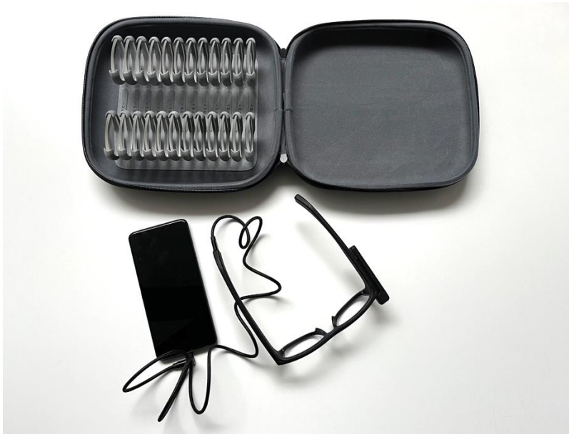
Fig. 91. Pupil invisible eye tracker connected with smartphone
