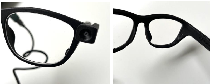
Fig. 92. Front camera (left) and back camera (right) of Pupil invisible eye
