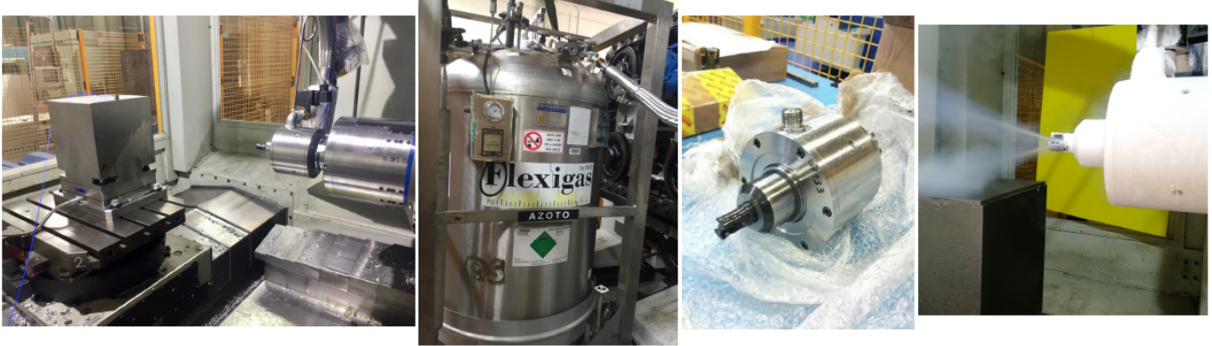
Figure 6.2.1: Experimental equipment, from left to right: Mandelli M5 horizontal spindle MT and workpiece mounted on dynamometric table, LN2 Dewar, Prototype spindle, working assembly
