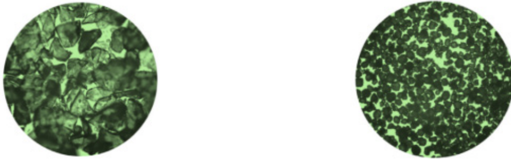
Figure 25. Two different mesh of luminescent powder doped into cement-based materials, case n°6. Reprinted from Construction and Building Materials, 269, 121267. Wang, W., Sha, A., Lu, Z., Jia, M., Jiang, W., Liu, Z., & Yuan, D. Self-luminescent cement-based composite materials: properties and mechanisms. Copyright (2015), with permission from Elsevier
