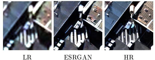
Figure 6: Test image, scale factor 4, ESRGAN "hallucination": an air-conditioning plant is super resolved as a car transformed into a car
