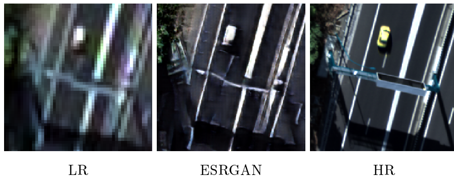
Figure 3.13: Test image from BD Merou dataset, scale factor 4. Second example of ESRGAN hallucination: a traffic sign is super resolved as a traffic line
