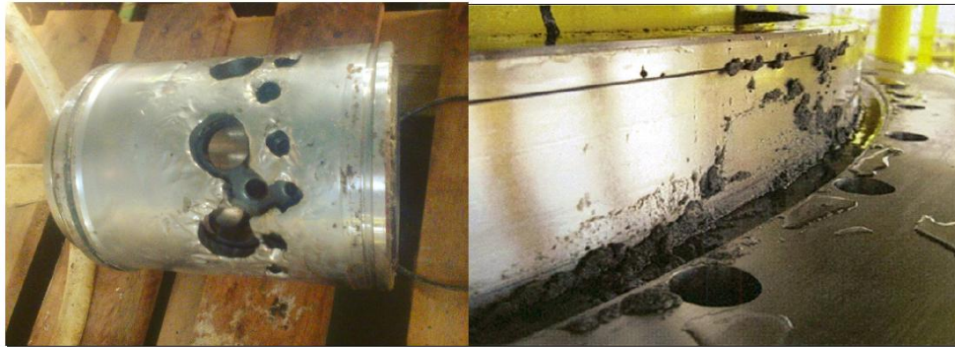
Figure 1.4: Effect of sand erosion in a gas transport pipeline (from [16]).
