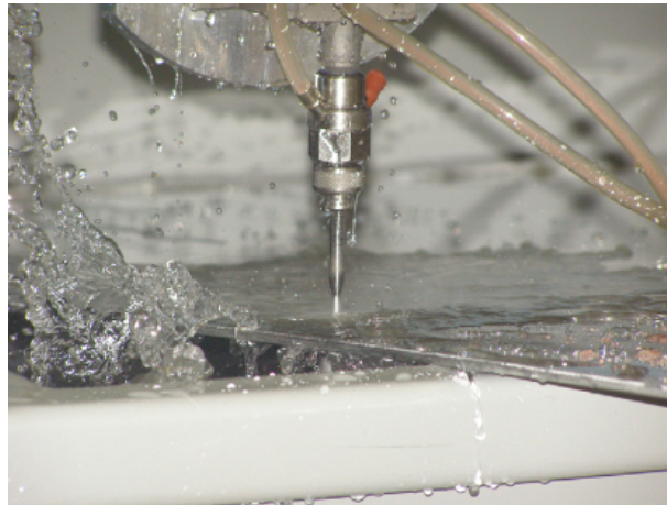
Figure 1.2: A close-up on a AWJM head (picture from [7]).
