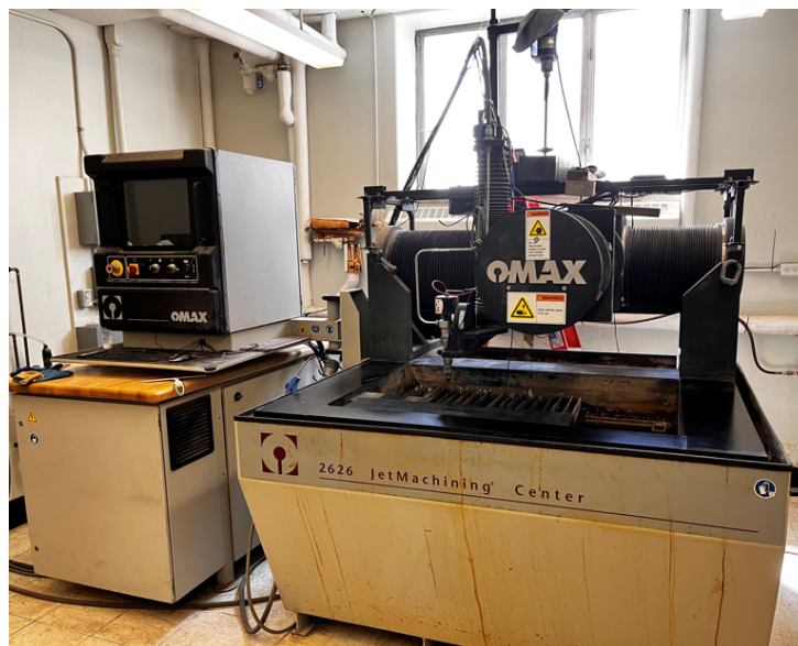
Figure 5.1: OMAX 2626 Jet Machining Center used for the experimental tests.
