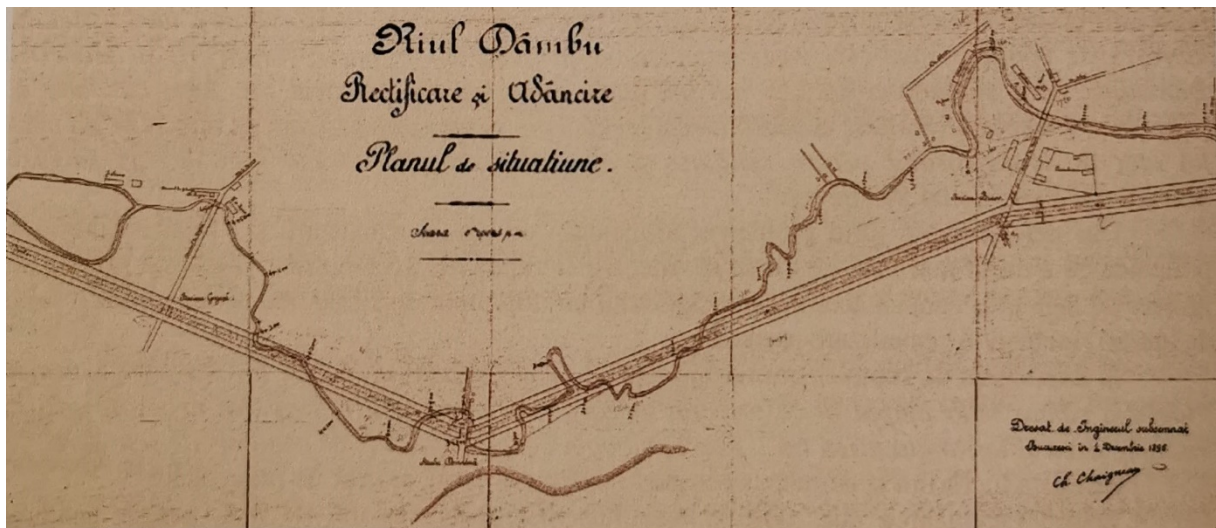
Figure 1 Plan of enginner Charles Chaigneaux for the regularization of Dâmbu stream 1896
