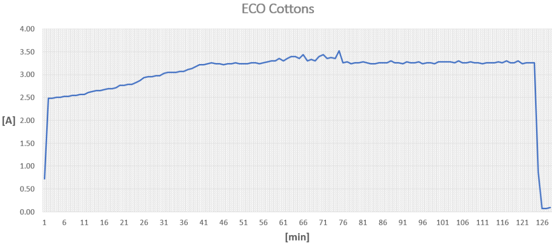
Figure 8.31. Current absorption for the ECO Cottons program
