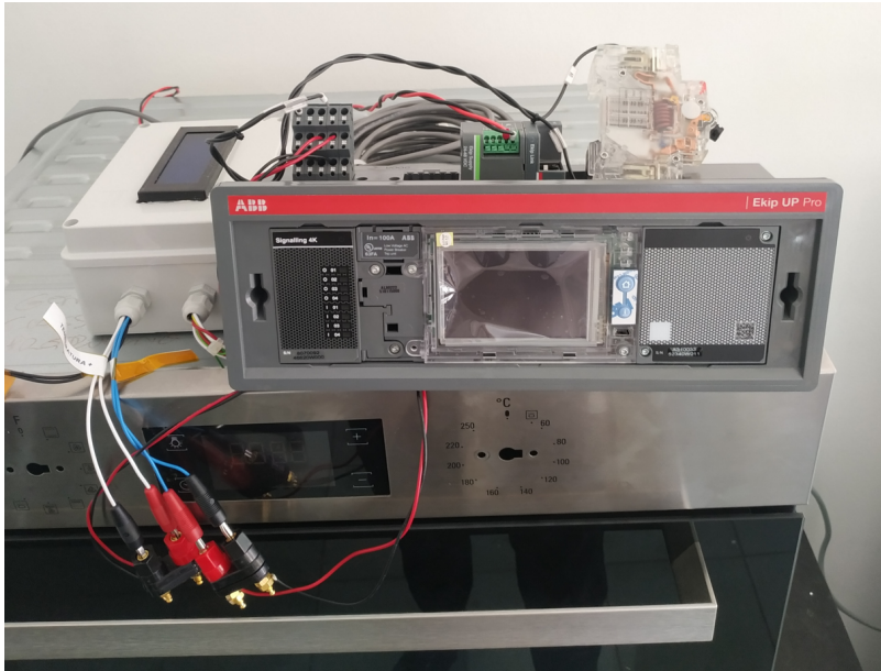
Figure 9.10. Picture of the instrumentation used to test the oven control logic
