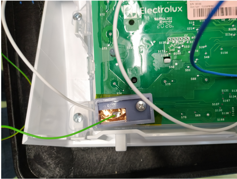
Figure 7.2. Picture of the modified capacitor
