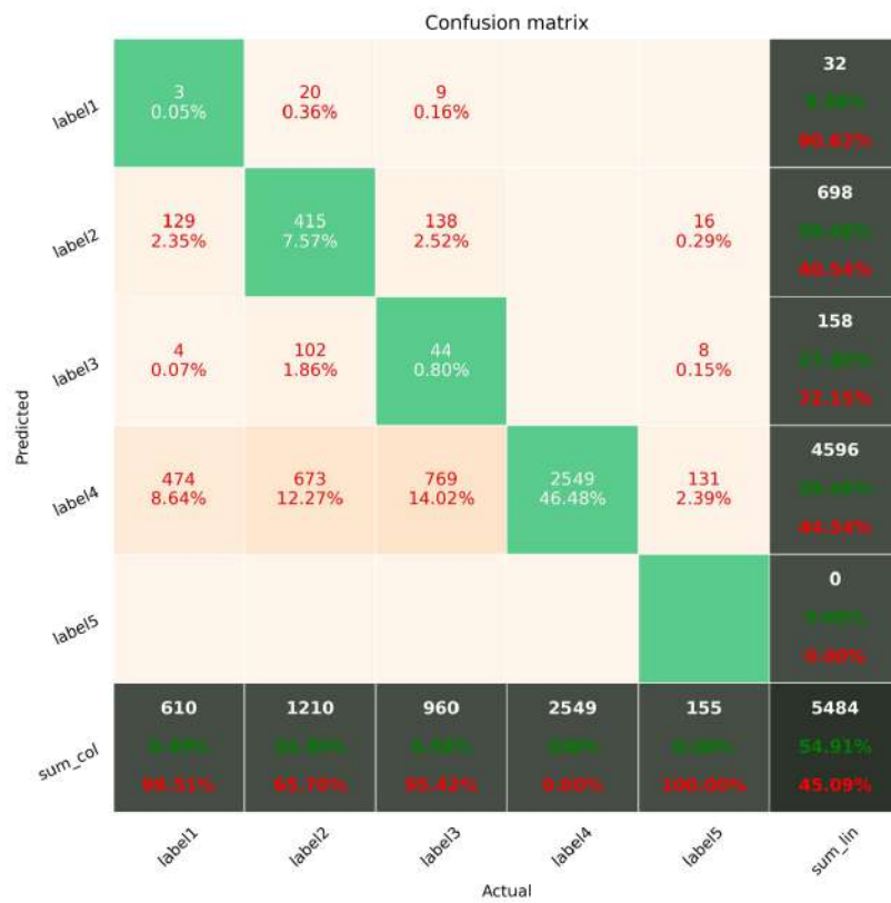
Figure 11.23: Ninth confusion Matrix for 15 Minutes Forecasting. The columns of this matrix shows the predicted label of the images. The rows of this matrix shows the Actual Label of the images. The prediction accuracy of the Ninth trial and is 54.91%.
