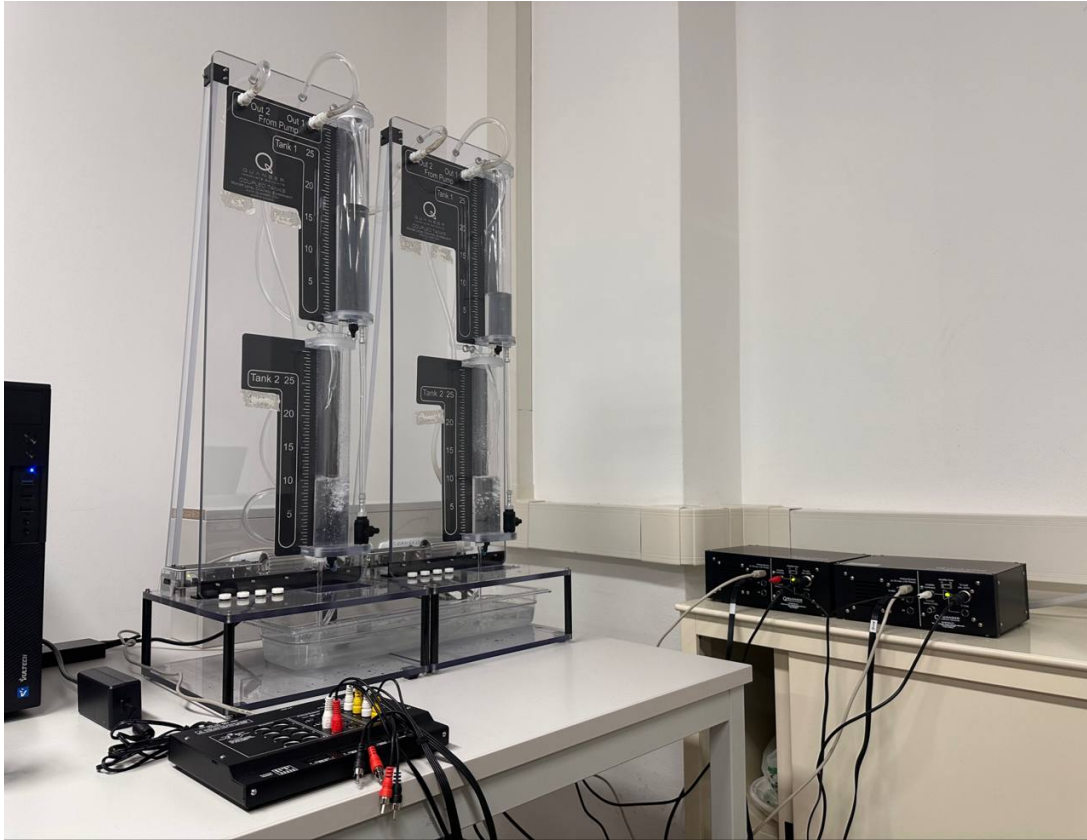
Figure 2.1: Lab-scale quadruple tank system in experimental setup.
