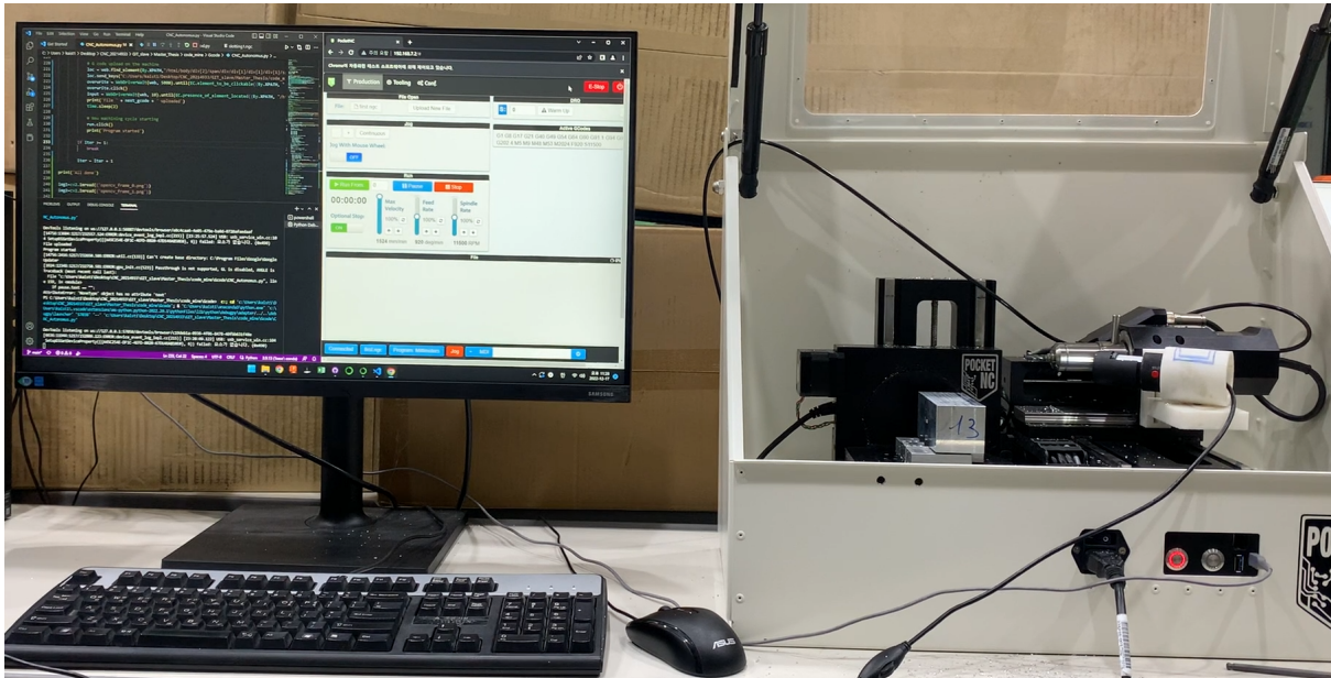
Figure 3.36: The final assembled system. There can be noticed the python script, the CNC controller web page, and the machine with the installed monitoring system.
