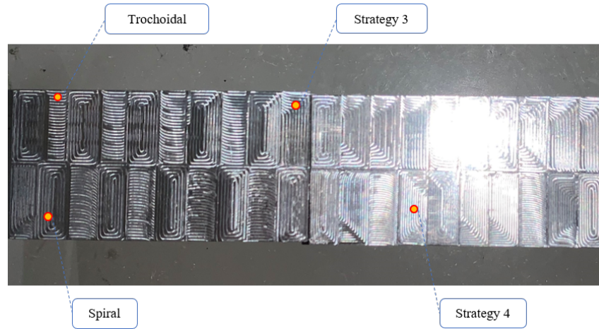
Figure 2.6: Two machined aluminium billets. The four different adopted machining strategies can be noted on the surface.
