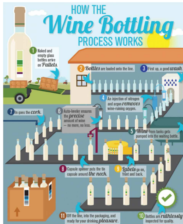
Figure 3. How the wine bottling process works/Sourced by visual.ly
